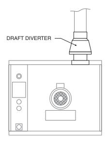
If the unit is to be connected to a direct flue, it is necessary that draft diverter be installed to insure proper ventilation.
